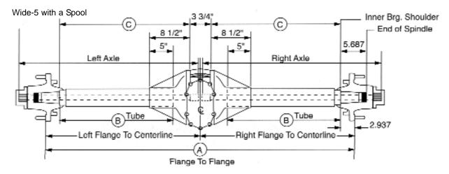
Note that above figure and corresponding measurements below are for a centered rear.
